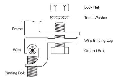
Figure 7: Installation Methods
