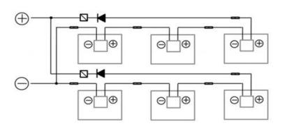
Fig.10-3 Parallel-series Connection
