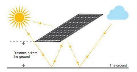
to install the module at a height from 0.5m to 2m. See Fig. 7-2.
