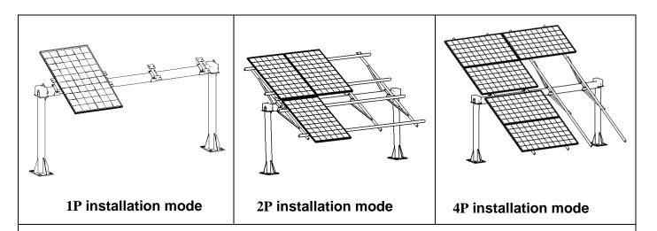
Risen module can be installed and used on the tracking system, and the installation hole position or clamp position shall be selected according to the design of the support system. Please refer to section 8.1,8.2 and 8.3 for details;
